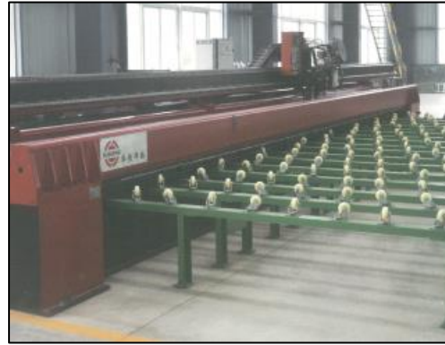
(P+T) Automatic Welder
